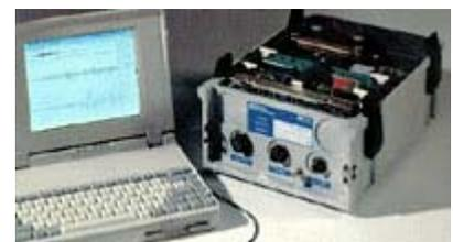
In order to provide the greatest flexibility in data storage, retrieval and communications, two fully compliant PCMCIA card slots are provided that support a wide variety of nonproprietary memory cards, hard disks and modems. This allows users to easily configure the K2 for their specific applications. Developed for Microsoft Windows™, QuickTalk® and QuickLook® software provides a user-friendly environment, making system setup, communications and rapid data analysis quick and easy.
